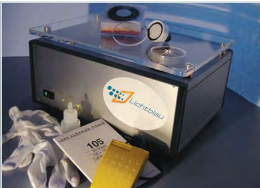
Figure 3. The SurveNIR spectrometer, which is controlled by a computer (not shown). The paper is rested on the top plate above the spectrometer case and measured at the lighted star point. Light exposure is only one second for a measurement. A book holder for safe handling of bound material is available.
