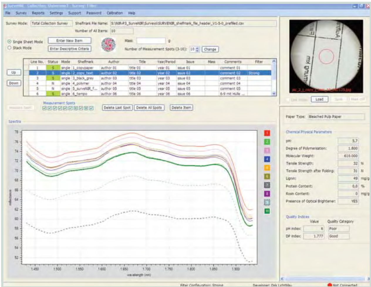
Figure 2. Screen output from SurveNIR, showing the measured NIR spectrum, the data gathered for each item, an image of the measuring spot (live video view; the red circle marks the measurement spot, an image can be saved with each spectrum), the derived chemical and physical properties of the paper, and the quality indices including quality categories.
