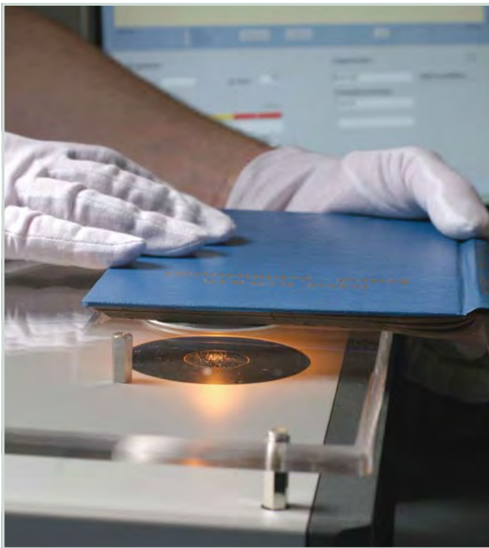
Figure 1. The SurveNIR instrument for non-destructive evaluation of paper chemical and mechanical properties for collection surveying, based on chemometric evaluation of NIR spectra.
