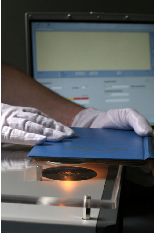
Figure 1: The SurveNIR instrument for non-destructive evaluation of paper chemical and mechanical properties for collection surveying, based on chemometric evaluation of NIR spectra.
