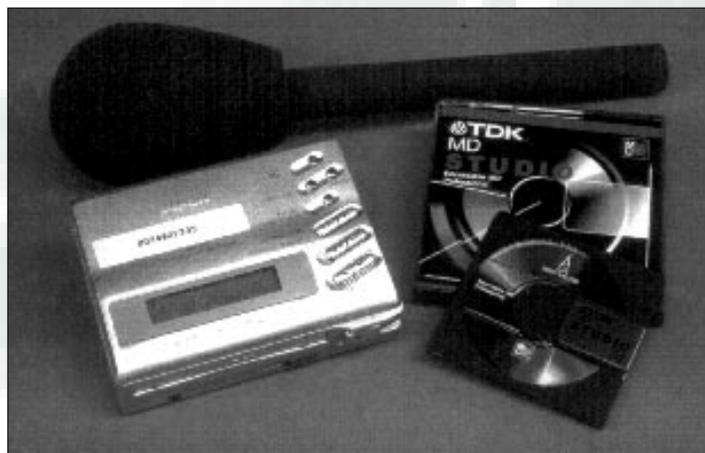
overtaken conventional CD. MiniDiscs are 64mm in diameter and come in a 68x72mm plastic case. The pre-recorded version is single-sided and is manufactured using similar digital technology to conventional published CDs. The recordable version is double-sided and relies on digital magneto-optical technology. As on the CD-R format, 74 minutes of stereo
